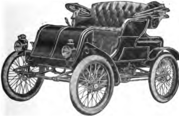
FIG. 60. —A Winton Touring Carriage, 1901 Model. This is one of the several excellent types of American motor carriage using a hand wheel for steering.
